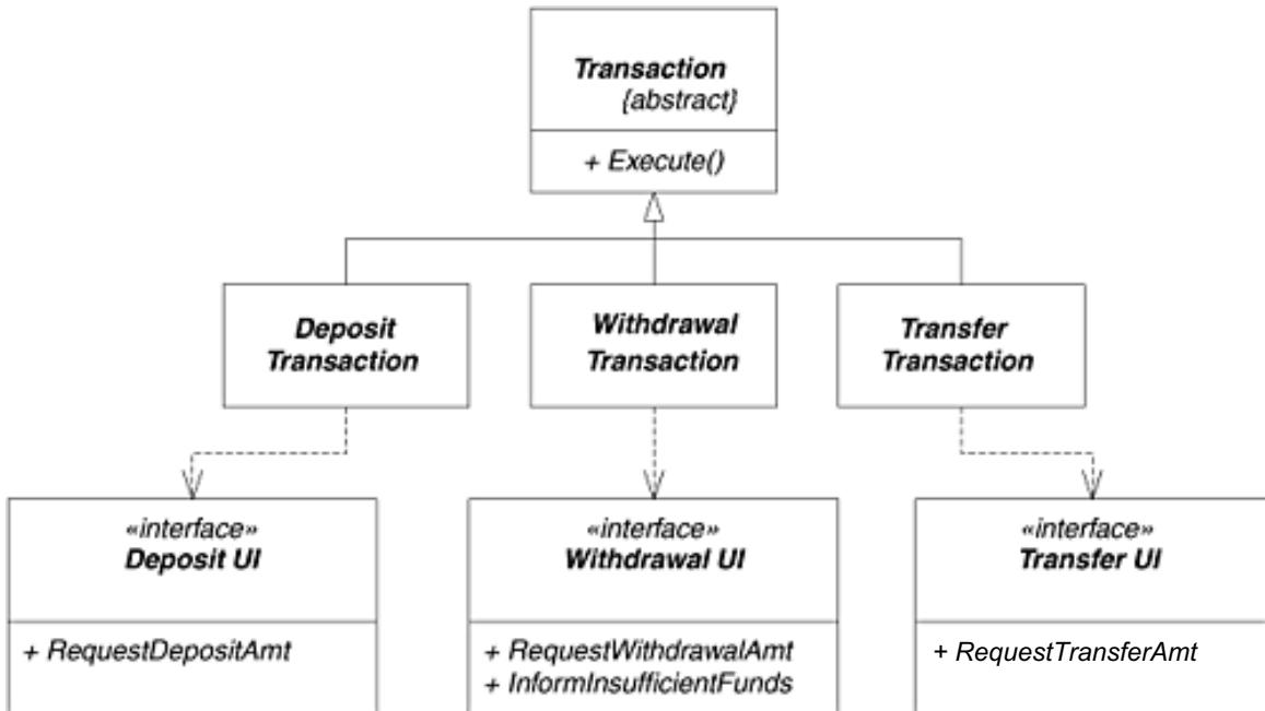
An alternative design: Decompose the bloated interface into multiple, separate interfaces
